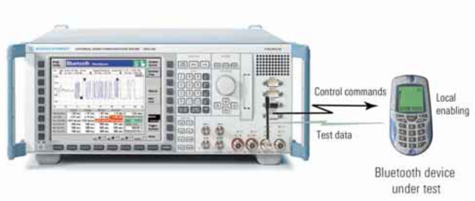
The device under test can be connected to the CMU200 via a RF coupler (antenna) or a cable
